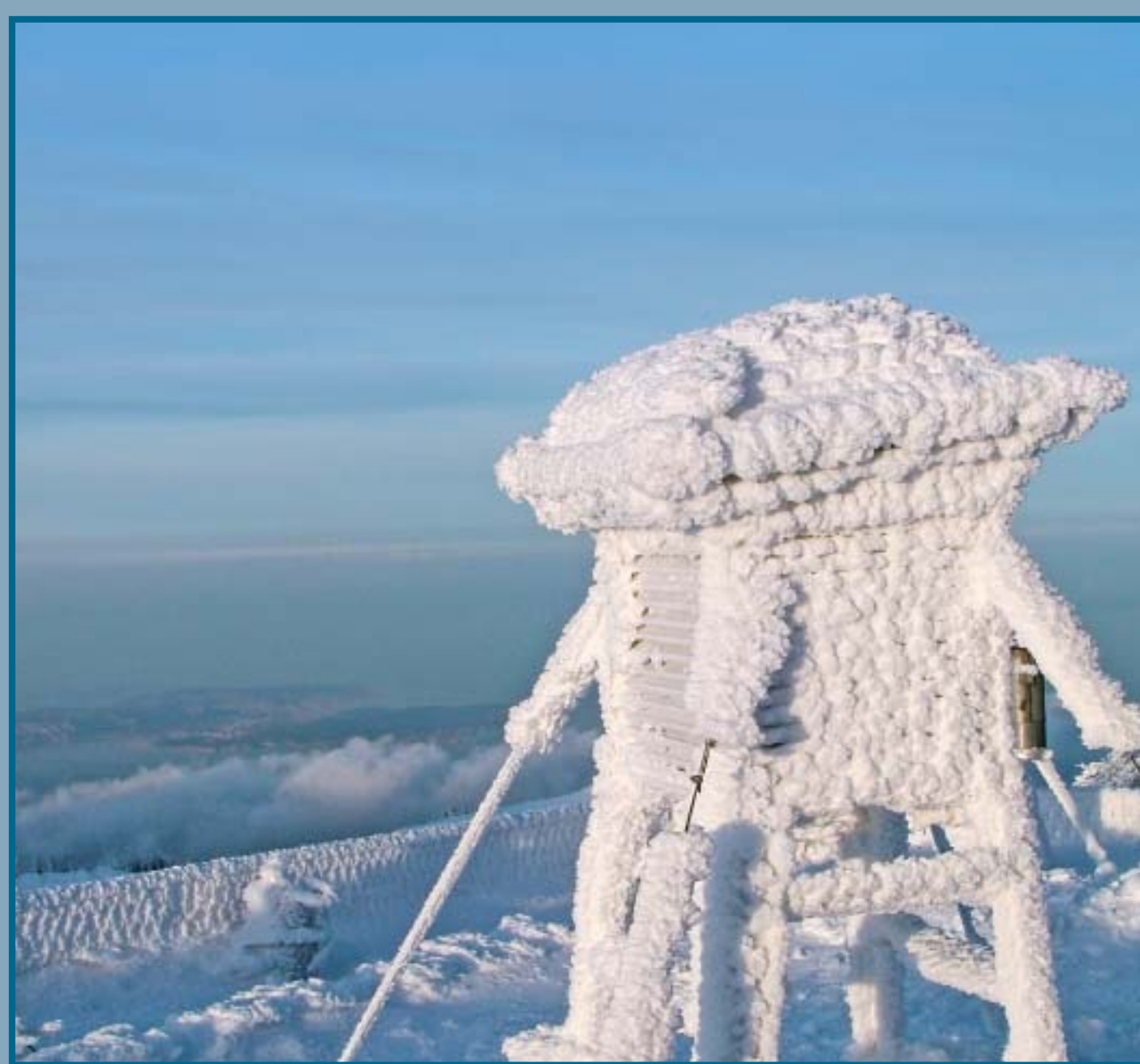
Meteorološka kućica okovana snijegom i injem. Meteorological screen bound with ice and rime.
